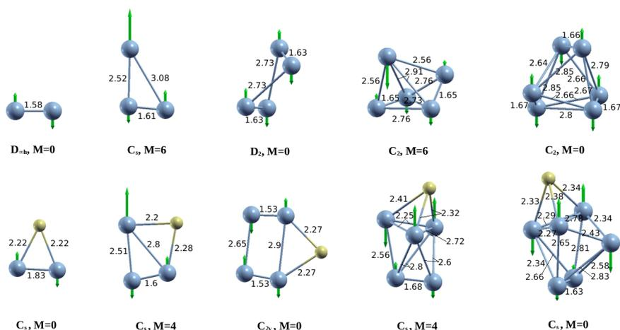
Figure : ground-state structures of neutral Cr<sub>n</sub> and Cr<sub>n</sub>S clusters with their symmetry and magnetic moment
